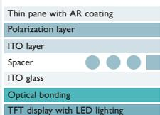
The GFG touch combines the proven, pressure-based analog resistive touch technology with a high-quality glass design. As a result, it is best suited for harsh ambient conditions. The device can be operated with fingers, gloves, stylus pens or any other object, without causing damage.
