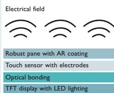
A transparent ITO layer underneath the glass cover, consisting of touch sensors, projects a uniform electrical field that extends through the glass to the user. The operator panels with PCAP touch technology support multi-touch functions and gesture control.
